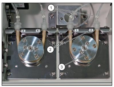
Figure 2.7 MID Standard Roller Pump
