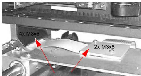
Figure 6-152 Flex cable fixtures
