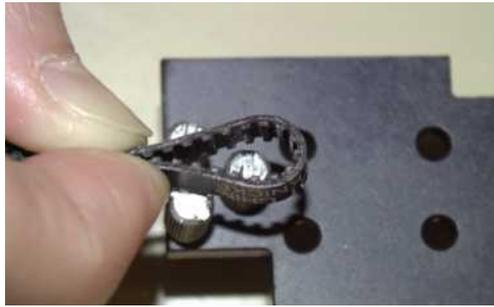
Figure 6-160 Installation of the Y-belt
