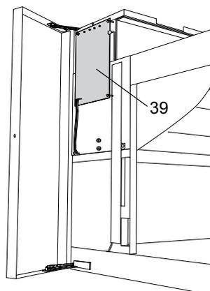
The Optibo is located in the left service compartment. On its rear side it holds the CU board and, plugged into latter, the X-DC-Servo board which controls the X-motor(s) for LiHa and RoMa.
