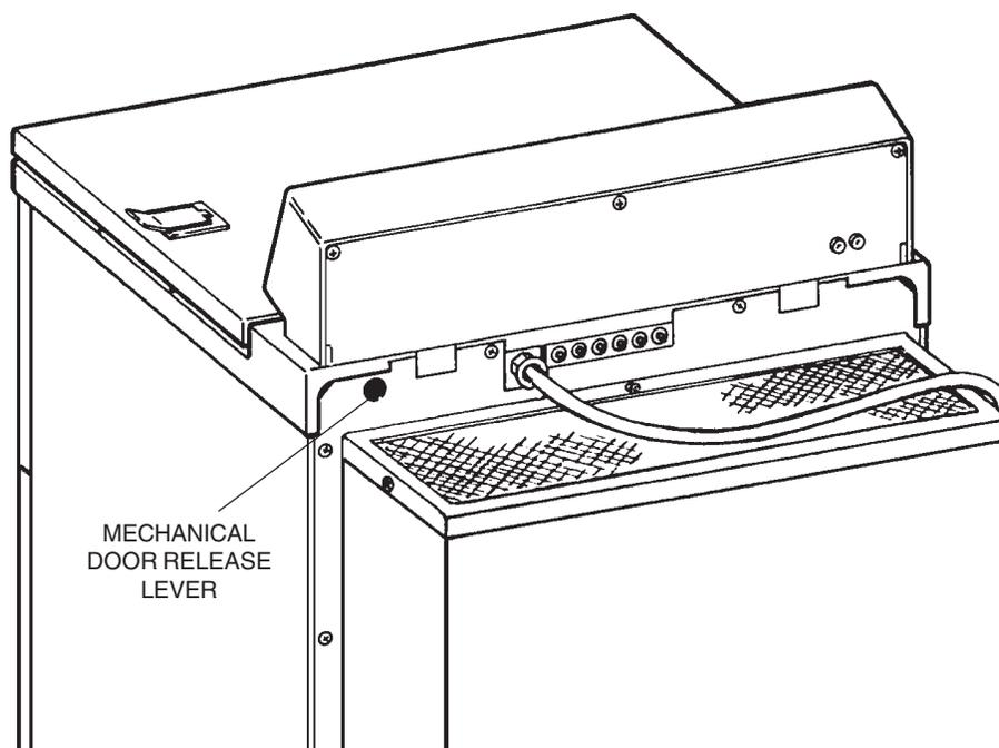
Figure 5-1. Location of Mechanical Door Release Lever
