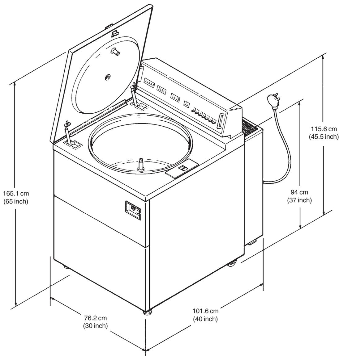
Figure 2-2. Centrifuge Dimensions
