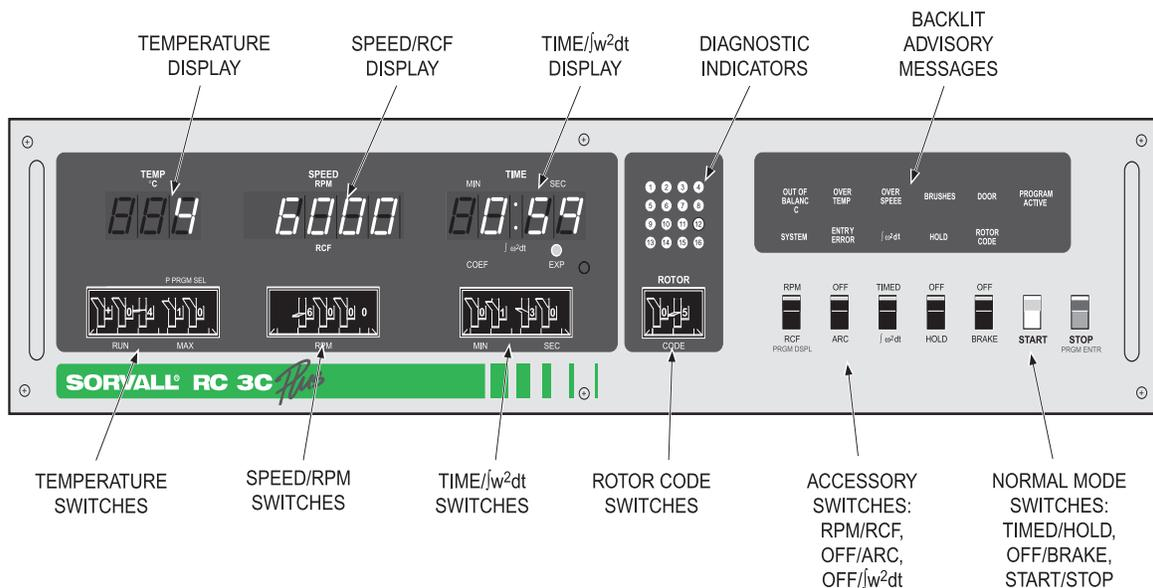
Figure 3-1. RC-3C PLUS Controls, Indicators, and Displays
