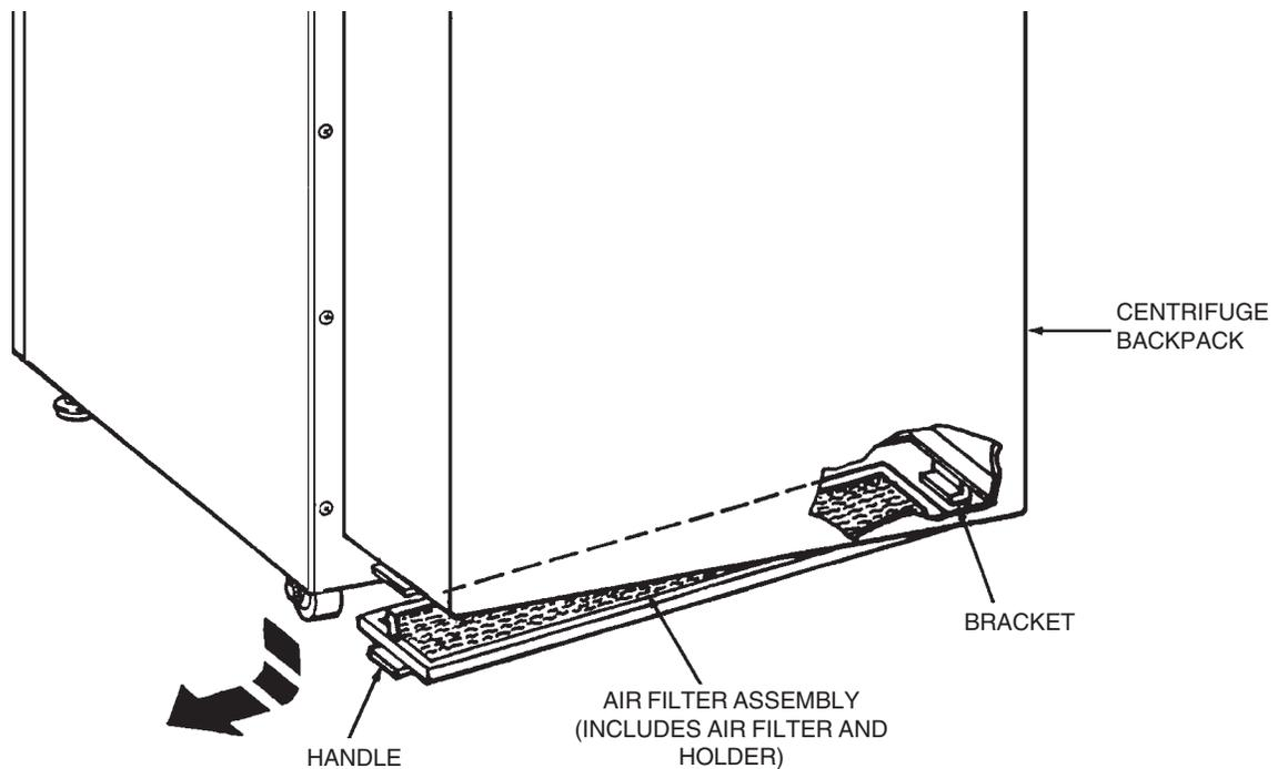
*Figure 5-2. Air Filter Assembly Removal*
